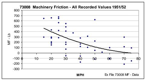
The incidence of negative MF outcomes clearly increases as a function of speed. Merchant Navy class 35022 showed similar traits, although the slope was less marked, the magnitude and frequency of negative outcomes was greater.
